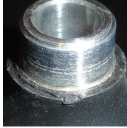
Figure 1: Problematic rubber-to-metal bonding (after destructive peel-back)
